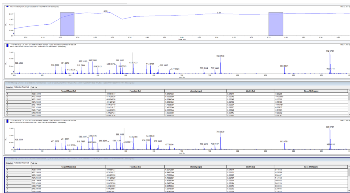
Figure 9-15 Reference Table Verification for MS Before Calibration
