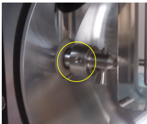
Figure 2-1 Set Screw for the Ion Source Baffle
